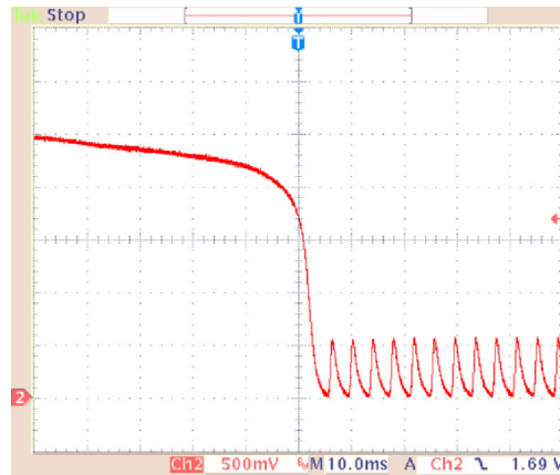
Fig. 10. Screenshot (oscilloscope) of high- B -SS to LC transition caused by decreasing Q at 0.64 for a single Repressilator circuit with QS feedback. Protein B voltage shown. Parameters: n = 3 , \alpha = 190 , \kappa = 10 , R_{hill} = 2.7 \text{ k}\Omega .
