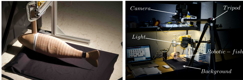
(a) Robotic fish including a silicone-rubber-based skin
