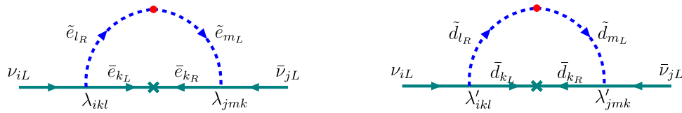
Fig. 5 One loop diagrams contributing to the neutrino mass: (left) with \lambda couplings and (right) with \lambda' couplings
