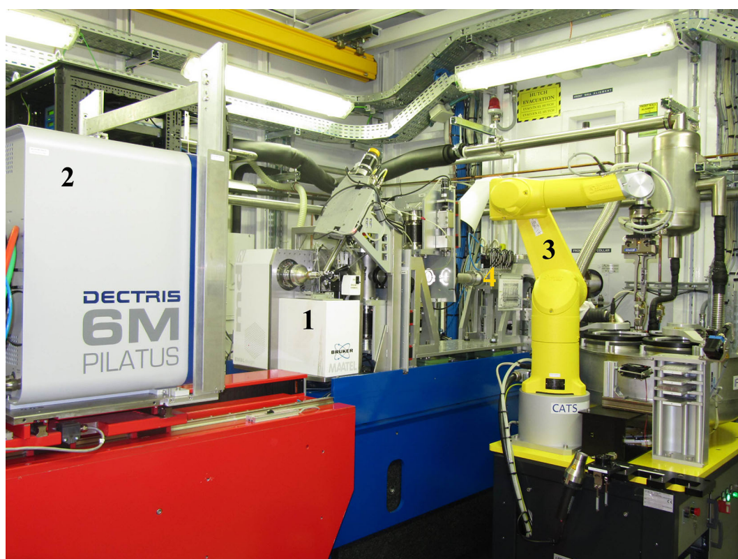
Fig. 5. End-station of the BL13-XALOC beamline dedicated to macromolecular crystallography. The main elements are the diffractometer (1), the pixel-array detector (2), the automatic sample changer (3), and the beam conditioning elements (4).
