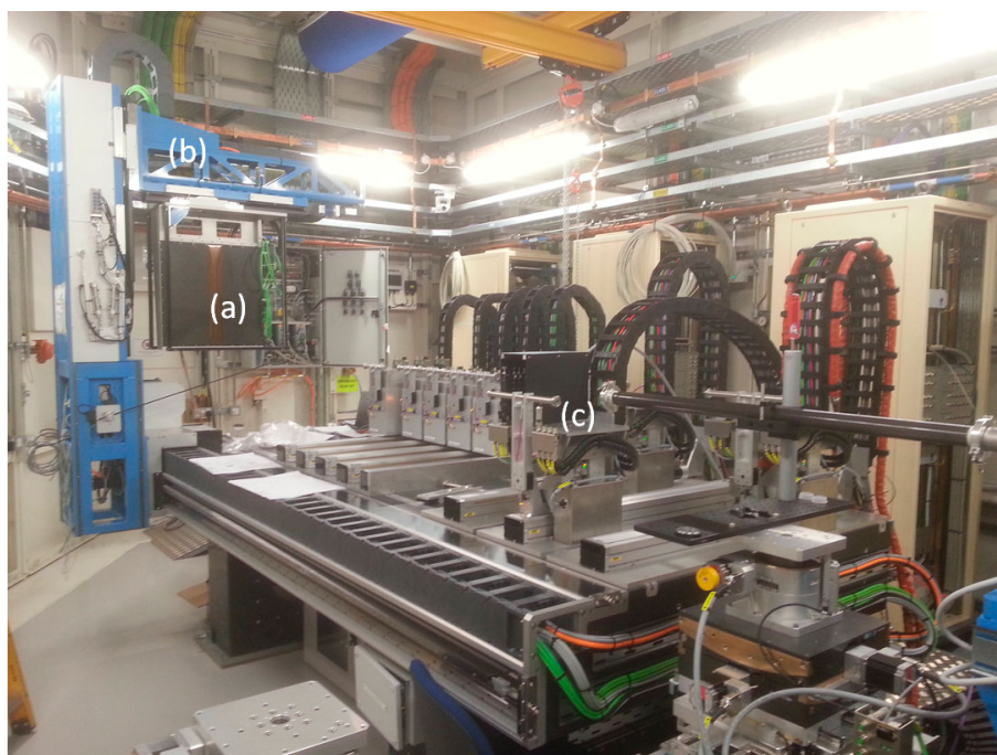
Fig. 14. The long duration experiments hutch (EH2) of beamline I11 during the final stages of equipment installation: (a) Pixium area detector; (b) detector translation stage; (c) sample stage.
