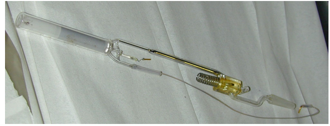
Fig. 1. One miniaturized proportional counters (MPC) handcrafted for Gallex/GNO [21].
