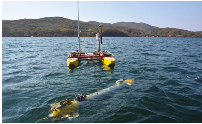
Fig. 5. Maneuvering of the ASV with an acoustical beacon and a DGPS-aided system in the vicinity of the AUV.
