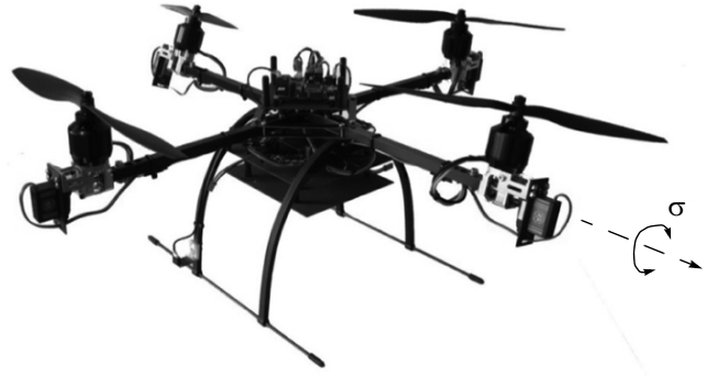
Fig. 1. Image of the actually built quadcopter with tiltable rotors.
