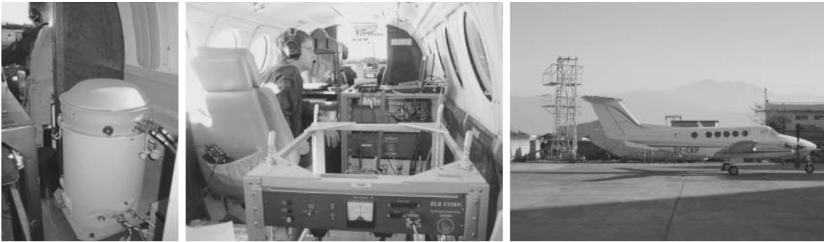
Fig. 4. Gravimeters used: Chekan-AM (left), L&R-S34 (center), both installed in King Air aircraft (right).
