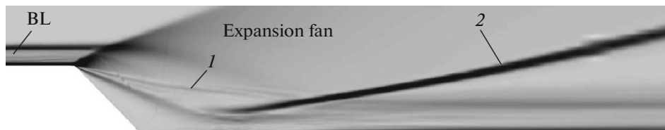
Fig. 37. Calculation of EWT flow pattern around tandem steps.
