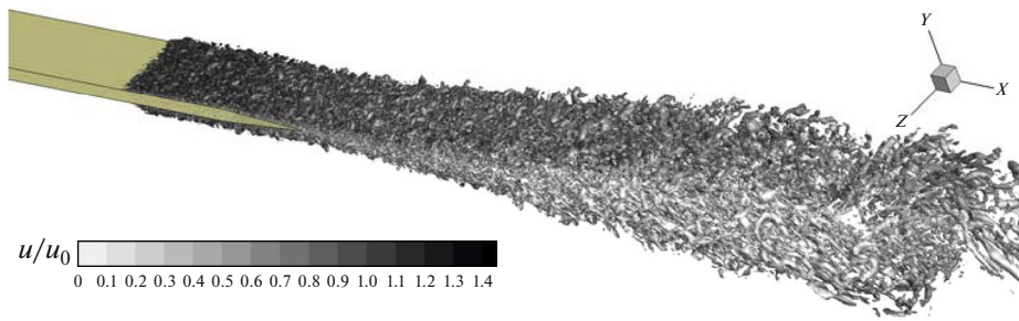
Fig. 8. Isosurface of swirl quantity \lambda (second eigenvalue of velocity gradient tensor) colored by streamwise velocity.
