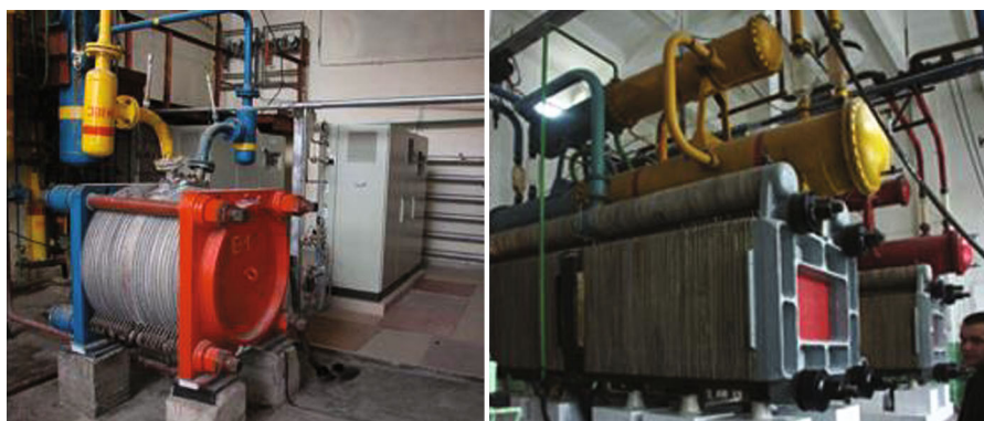
Fig. 11. (Color online) Uralkhimmash modules of electrolysis of types SEU (SPP) (a) [80] and FV (PhR) (b) [81].
