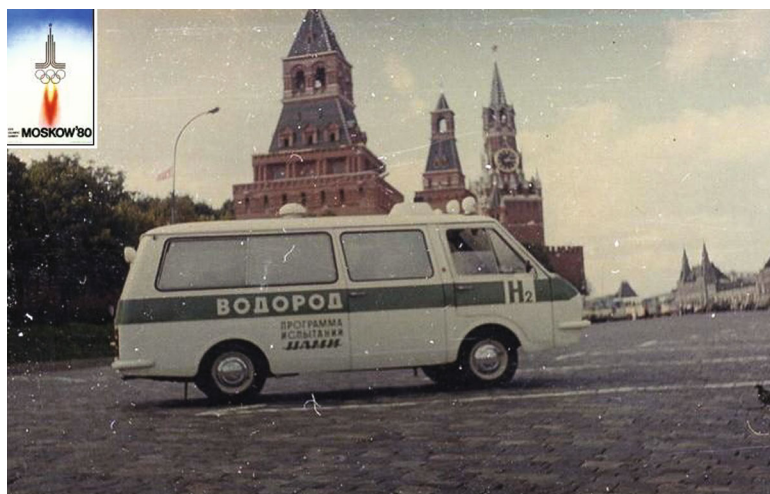
Fig. 3. (Color online) Minibus RAF running on hydrogen and gasoline (1979).
