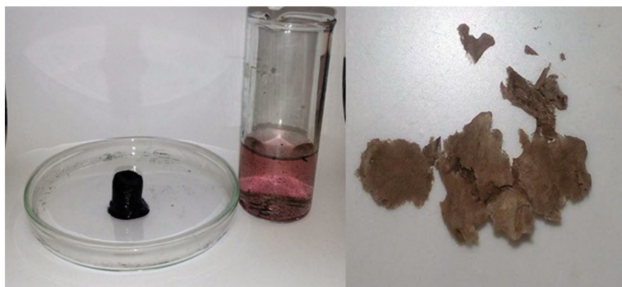
Fig. 1. (Color online) A sample of the rGO–AuNPs hydrogel and the remaining solution from the autoclave.
