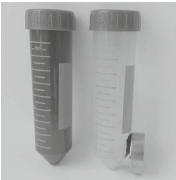
Fig. 5. Illustration of the action of a constant magnetic field on an aqueous Fe 3 O 4 @TEOS/MPTMS@Au coll dispersion.
