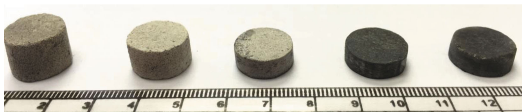
Fig. 6. (Color online) Samples of ceramic zeolite-based materials fabricated by the SPS synthesis at temperatures from 700 to 1100°C (increment of 100°C).
