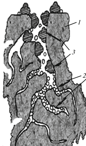
Fig. 2. Character of MBT sorption with a CNF sample: (1) CNF agglomerate, (2) monomolecular MBT sorption in micro- and mesopores of the agglomerate; (3) polymeric MBT sorption in macropores of the agglomerate.
