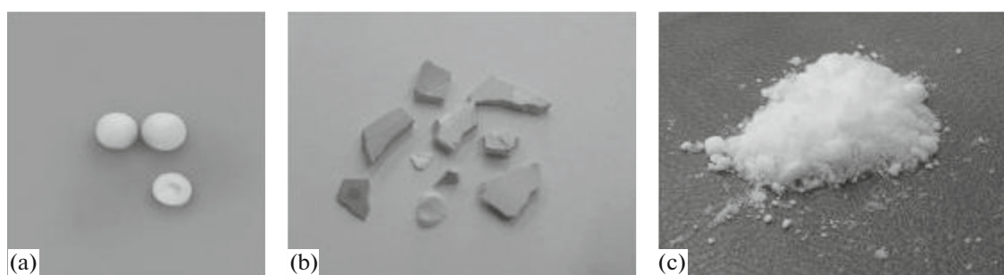
Fig. 1. View of initial SiO 2 carriers: granules—GR (a), opal—OP (b), ultrafine (Aeroxide)—UF (c).
