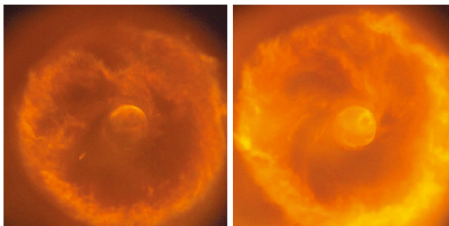
Fig. 11. Self-ignition center in the center of the reactor at different points in time. The difference between frames is 0.1 ms. Blend, 40% H 2 + 60% air. The temperature of the reactor walls is 558 K.
