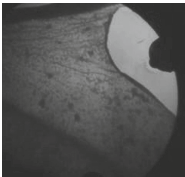
Fig. 6. Microphotograph of a film of modified lubricating composition ( K_{\text{mag}} = 220000\times ).
