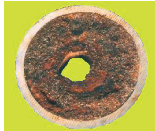
Fig. 17. Appearance of cross section of the pipe with paraffin crystals deposited on walls.
