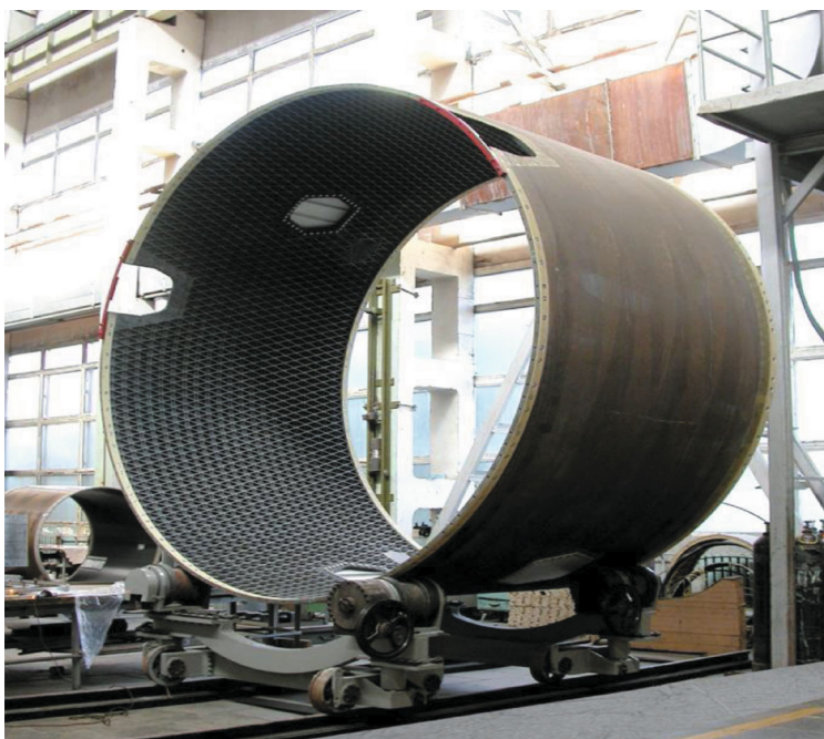
Fig. 10. Lattice structure of the lower coupling section of a Proton-M carrier rocket made of the carbon-fiber-reinforced plastic with the organic-fiber-reinforced-plastic outer shell. The section diameter is 4100 mm, and the height is about 3000 mm.
