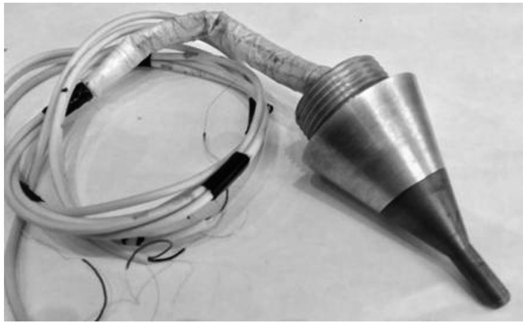
Fig. 7. Heat flux density sensor DTP-GD-2.1.
