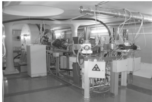
Fig. 3. SS-18/9M cyclotron with remote targets.
