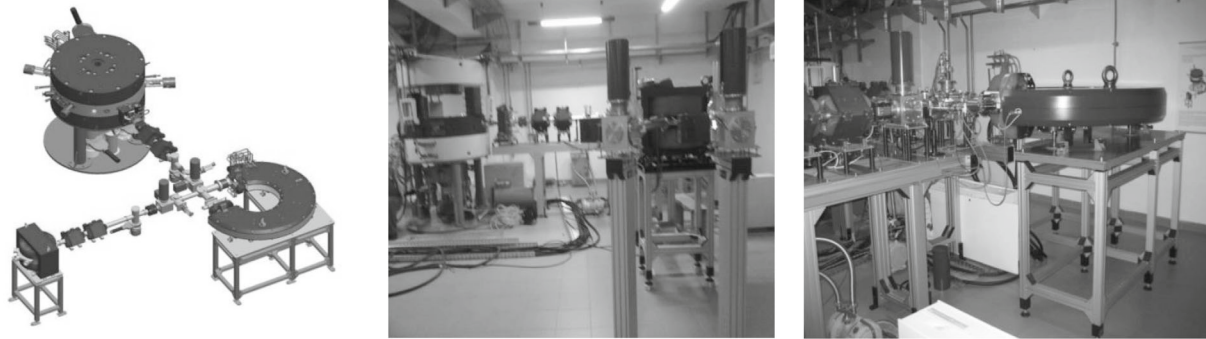
Fig. 1. SS1-3 cyclotron system with the beam-shaping and -transport channel.
