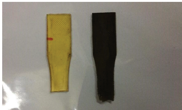
Fig. 10. Cross-linked polymer (right) and linear polymer (left).
