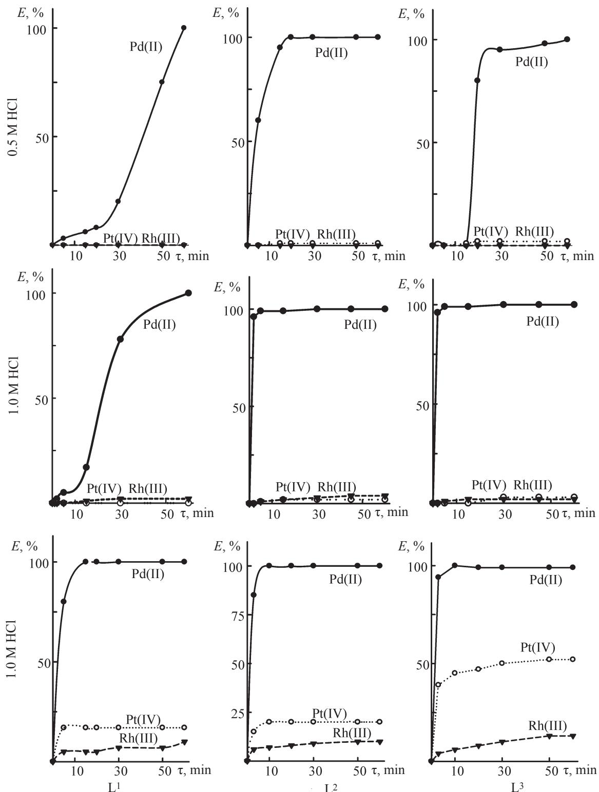
Degree of recovery  $E$  of palladium(II), platinum(IV), and rhodium(III) with reagents  $L^1$ ,  $L^2$ , and  $L^3$  from solutions simulating solutions from the refining process after separation of the palladium concentrate as a function of the aqueous phase acidity and phase contact time  $\tau$  ( $20^\circ\text{C}$ ,  $10 \text{ g L}^{-1}$  NaCl,  $A : O = 10 : 1$ ,  $c_L = 0.25 \text{ M}$ , chloroform diluent).
