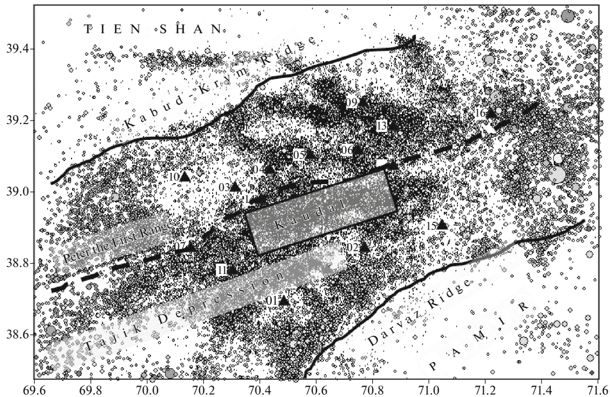
Fig. 1. Tectonic elements and seismological observation system at Garm geodynamic test site of CGE IPE USSR Acad. Sci. Triangles with numbers are seismic stations. Small circles are epicenters of earthquakes with M \geq 0.5 that occurred from January 1, 1955 to March 31, 1992. The box in center is Kaudal local region (LR) considered for studying time variations in b -value with depth.
