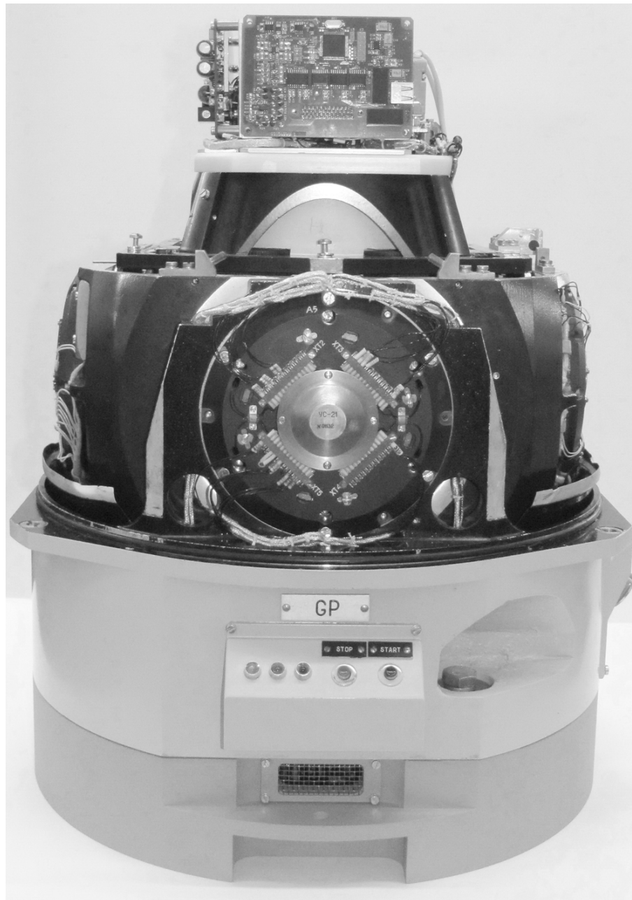
Fig. 1. The exterior view of the Chekan-AM gravimeter (Shelf-E modification).
