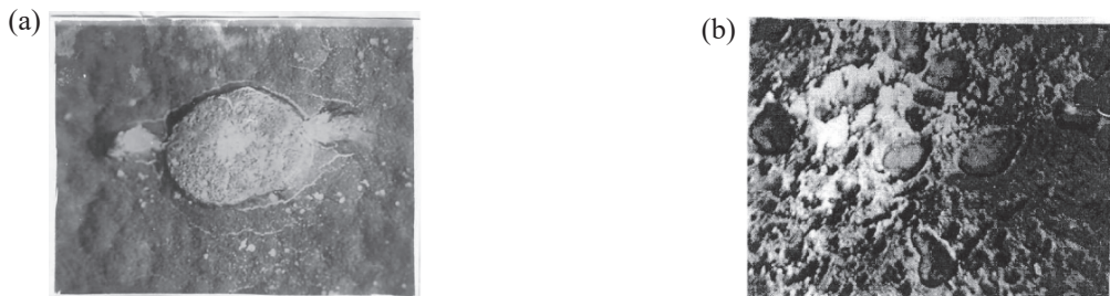
Fig. 4. (a) Microstructure of the U–Zr alloy with the inclusion area (magnification \times 200 , secondary electrons); (b) inclusion microstructure (magnification \times 1000 , absorbed electrons). The dark areas are the phase of the basic composition, the light areas are the phase enriched with zirconium, tin and other elements.
