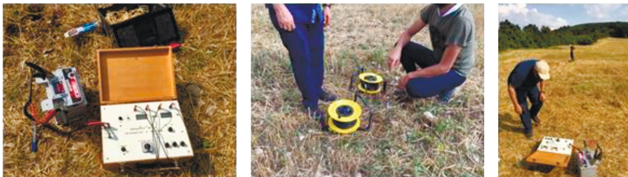
Fig. 5. Resistivity data acquisition by two electrodes array.
