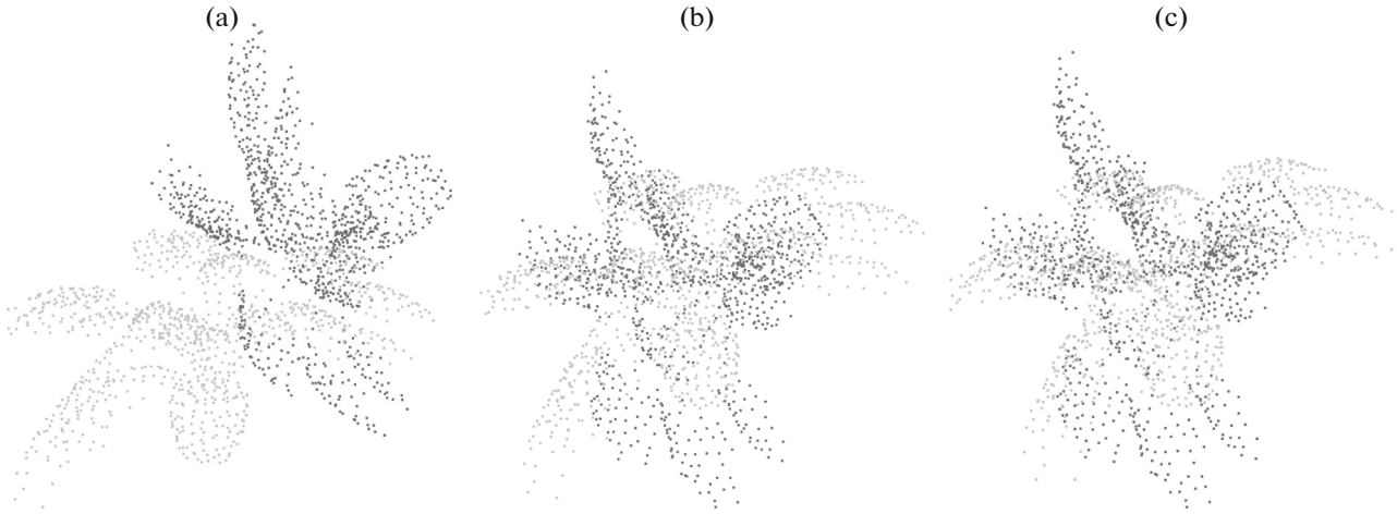
Fig. 10. (a) Point clouds: (gray dots) source and (black dots) target; (b) results of the CNN registration; and (c) result of the CNN + PtP registration.
