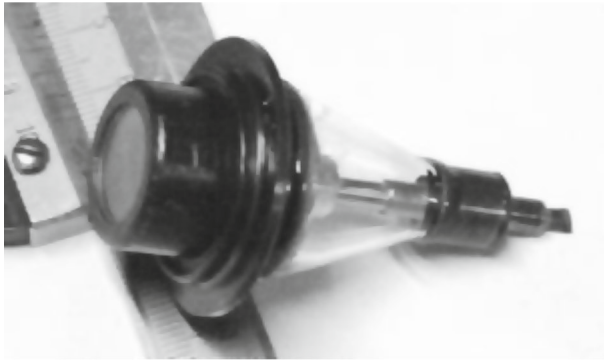
Fig. 3. Photograph of the X-ray tube with a glass insulator.
