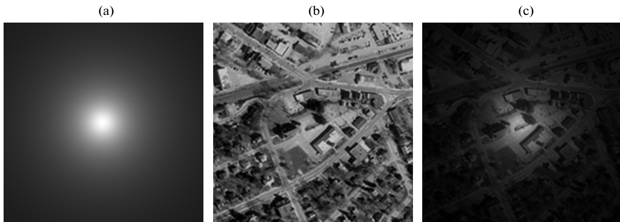
Fig. 10. (a) Function of nonuniform illumination with \tau = 5^\circ , \alpha = 245^\circ , and r = 0.3 ; (b) the original image; (c) the image distorted by nonuniform illumination and a white noise with a standard deviation of 1.
