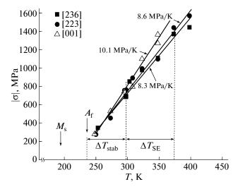
Fig. 2. Temperature dependences of the critical stresses of martensite formation in compression-strained Ni<sub>51.0</sub>Ti<sub>36.5</sub>Hf<sub>12.5</sub> single crystals oriented along [001], [236], and [223] directions:  $(\Delta T_{\rm stab})$  temperature interval of stress-induced martensite stabilization;  $(\Delta T_{\rm SE})$  temperature interval of SE.
