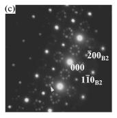
**Fig. 1.** Microstructure of as-grown  $Ni_{51.0}Ti_{36.5}Hf_{12.5}$  single crystals: (a, b) bright-field and dark-field TEM images, respectively; (c) the corresponding selected area diffraction pattern, zone axis is  $[001]_{B2}$ ; the dark-field image was recorded using the reflection indicated by the arrow in the diffraction pattern.
