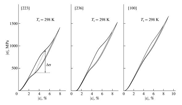
Fig. 3. Stress—strain curves  $\sigma(\varepsilon)$  measured at  $T_t = 298$  K in compression-strained Ni<sub>51.0</sub>Ti<sub>36.5</sub>Hf<sub>12.5</sub> single crystals oriented along [223], [236], and [001] directions.
