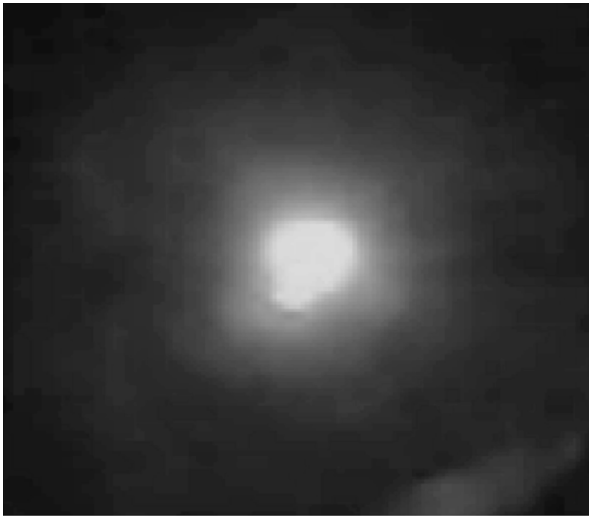
Fig. 1. Photograph of the glow of a nanosecond-discharge plasma in atmospheric-pressure air between electrodes made of polycrystalline chalcopyrite \text{CuInSe}_2 (the vertical size of the glow region is approximately equal to the inter-electrode spacing of 2 mm).
