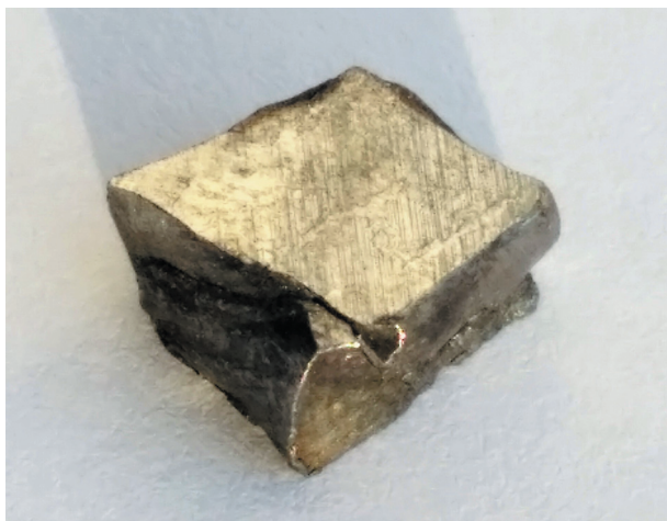
Fig. 6. Sample cracked after compressive strength test.
