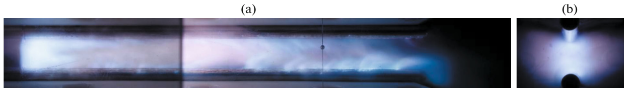
Fig. 5. The image of high-current discharge obtained by camera under long exposure time. (a) Side view; (b) front view. The cathode is bottom electrode. Nitrogen, P = 50 Torr, h = 30 mm, U_0 = 5 kV, I_{\max} = 25 kA.
