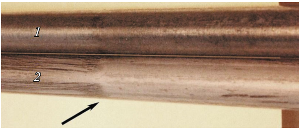
Fig. 14. The images of the working surface of the anode (1) and cathode (2) after a series of discharge starts. The arrow shows the place of a high-current discharge initiation. The sharp spikes initiating the discharge at this place are removed. The direction of the accelerated plasma movement is from left to right.
