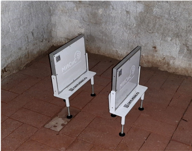
Fig. 1. Nuclear-photoemulsion detectors placed in the basement of one of the churches of the Holy Trinity Danilov Monastery.
