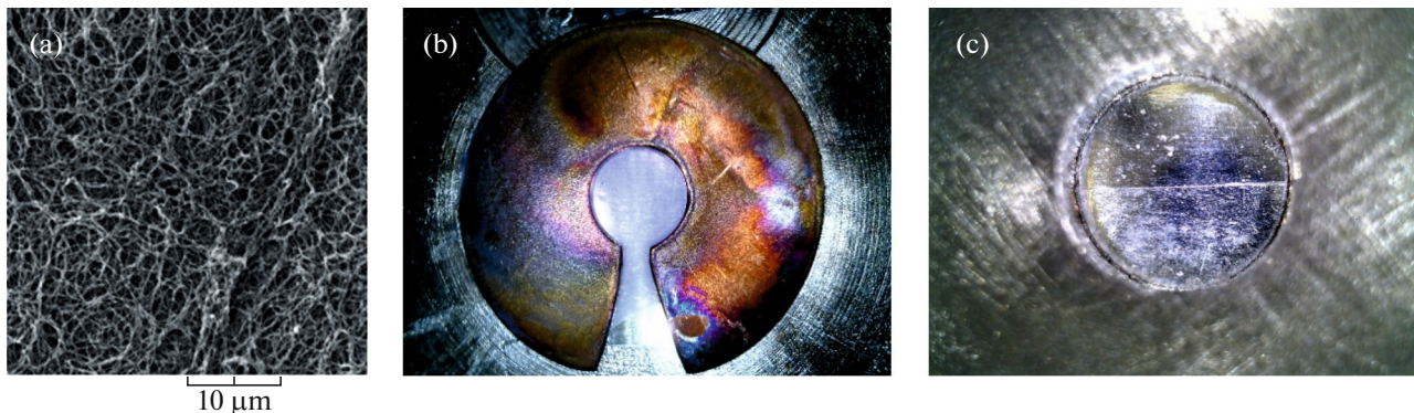
Fig. 2. Photographs showing (a) foam microstructure and (b, c) target viewed from the frontal (foam) and rear (profiled aluminum) sides, respectively.
