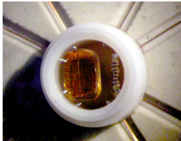
Fig. 3. (Color online) Sample (for calibration) and the manganin gage in an ampule with a hydrostatic medium.
