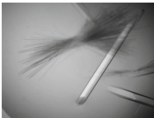
Fig. 1. Crystals of E. coli purine nucleoside phosphorylase grown by the vapor-diffusion technique using sulfate ammonium as the precipitant. The crystal length is 0.7 mm.
