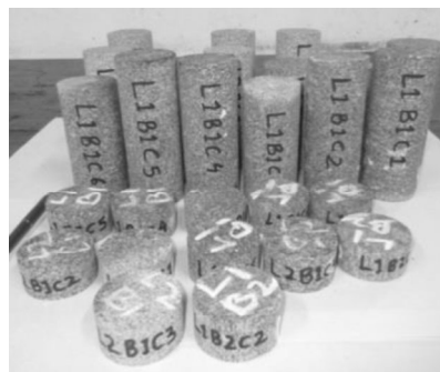
Fig. 3. Prepared rock samples as per ISRM standards.
