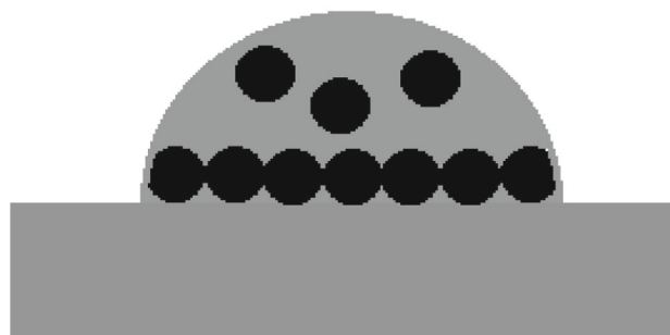
Fig. 9. The state of the adsorption layer of particles at the moment of meniscus fixation on a hydrophobic substrate.
