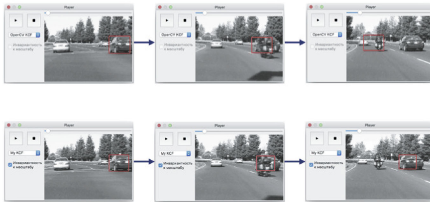
Fig. 6. Comparison of the operation of the standard KCF tracker (upper part) and the modified tracker with obstacle handling (lower part).
