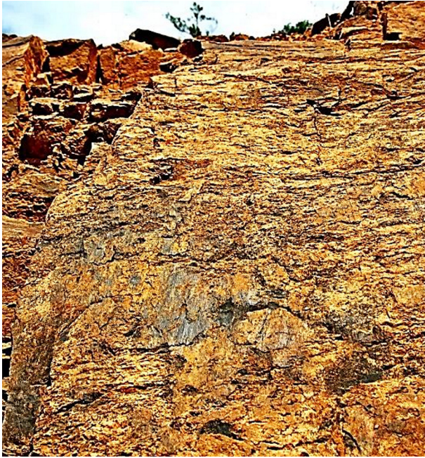
Fig. 3. Slickenside in the granite barrow pit (Petrov village) located in the Primorsky normal fault zone. Seen are subvertical slickenlines characteristic of normal faults with signs of weak chloritization as well as signs of highly intense metasomatic transformation and a thin film of frictional melting (vitrification), which indirectly indicate shallow depths of its origin, presumably during the Neogene-Quaternary period of formation of the Baikal Rift basin (photo by V.V. Ruzhich) (color online).
