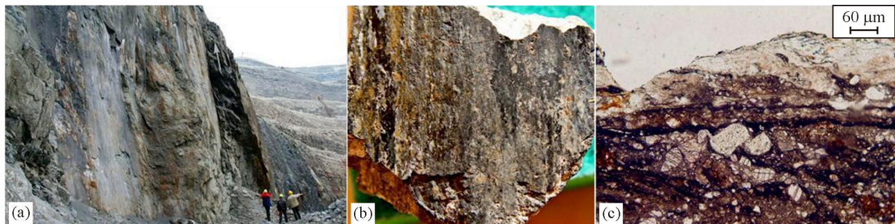
Fig. 9. Different-scale heterogeneities from a segment of the Vilyui fault zone (az. 50^\circ – 60^\circ NE): a—one of the large-scale slickensides in the ultradeep Udachny mine exposed at the depth 475 m; b—slip surface fragment containing a slickenside; c—polished section of the slickenside shown in Fig. 9b with two slip planes formed in different periods of coseismic slips (color online).
