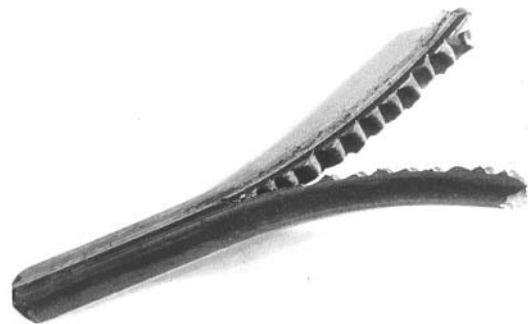
Fig. 5. Specimen of 37CrNi3MoVN steel failed on rolling [23]
