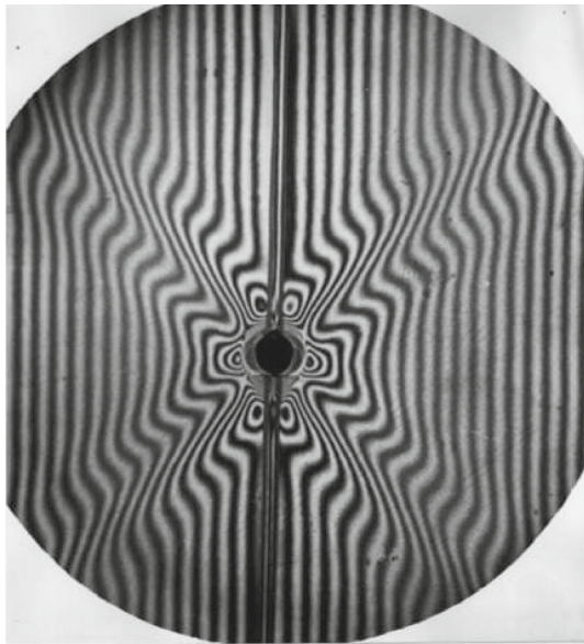
Fig. 1. Schlieren-interferometric image of the internal-wave field generated by a vertically vibrating cylinder with the diameter d = 1 cm in a fluid with a linear density profile.
