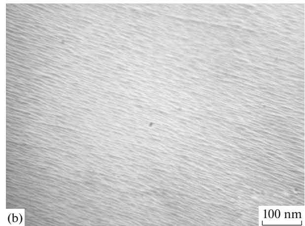
Fig. 3. Sapphire surface after ion polishing ( 2000\times magnification) at different \alpha angles: a — 70^\circ ; b — 30^\circ .
