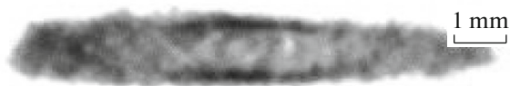
Fig. 3. Virtual cross section of the copper pulo from the analysis of a 3D model. Dark areas correspond to regions with greater neutron-beam attenuation coefficients and, presumably, are associated with patina. Lighter areas correspond to copper.
