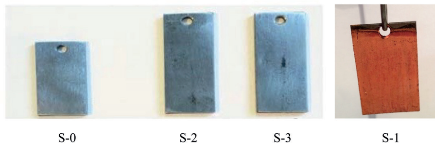
Fig. 1. Carbon steel samples exposed in the fuel oil-catalyst-air medium for 200 h: (S-0) initial carbon steel plate; (S-1, S-2, S-3) steel samples exposed in the fuel oil in the presence of K-1, K-2, and K-3 catalysts, respectively; 90°C; V_g/V_l = 0.4 ; [\text{H}_2\text{S}]_0 = 128 ppm; [\text{C}_2\text{H}_5\text{SH}]_0 = 72 ppm; [\text{kat}] = 300 ppm.
