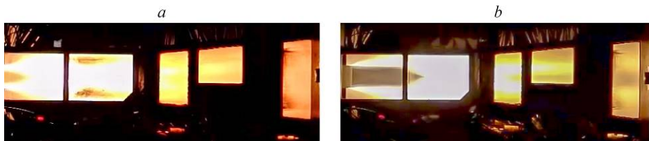
Fig. 15. Flame visualization for configurations with 90-degree (a) and 45-degree (b) fuel injection.
